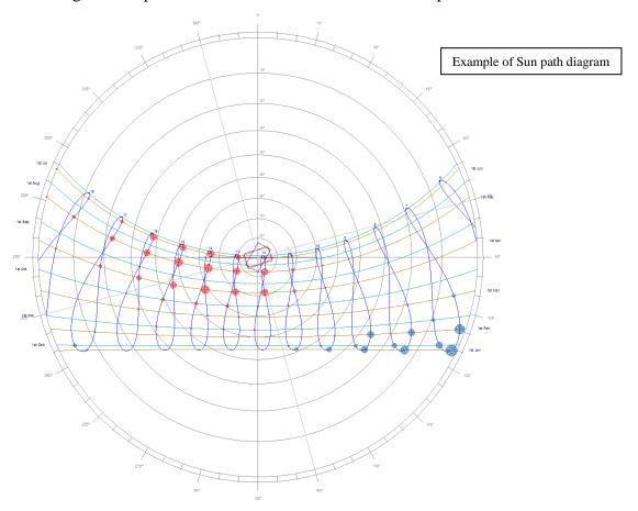
Similarly Humidity is also plotted on the Sunpath Diagram. This enables Students to know that all the white portion of Sunpath is comfortable for occupants and all the Red portion is to be avoided. This method also provides the intensity of the sun in the hot zone which guides the orientation of the building as shown in the figure above.
