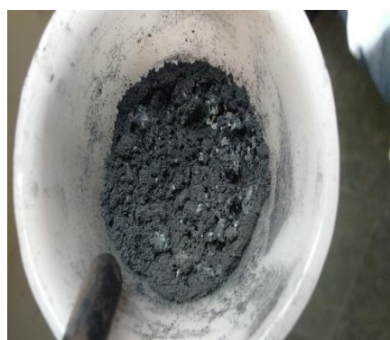
Figure 2. Spongy structure of expanded graphite after heat treatment
