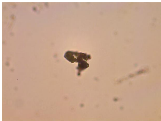
Figure 3. Optical microscope image of expanded graphite (route-I) under 50X magnification
