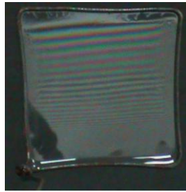
Figure 5: Interference on a Vertical Soap Film
