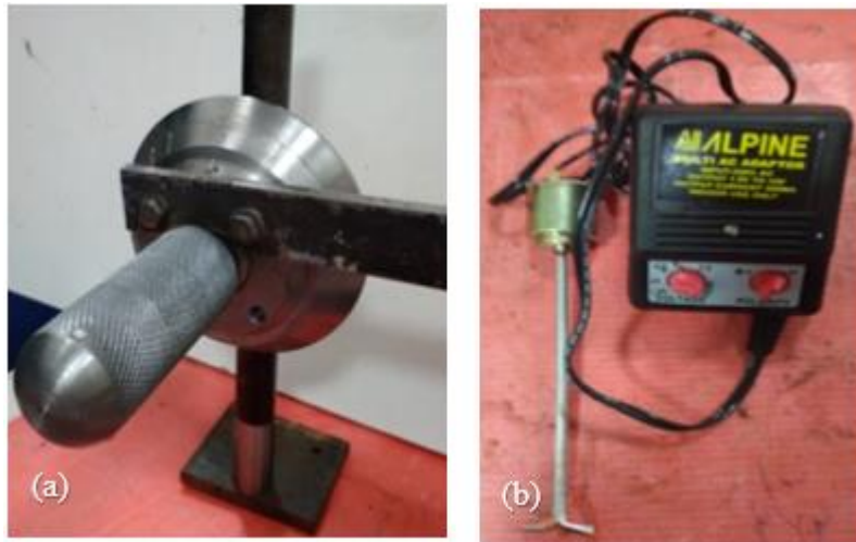
Figure 3.2 (a) welding torch angle change (b) Stirrer for mixing flux and carrier solvent
