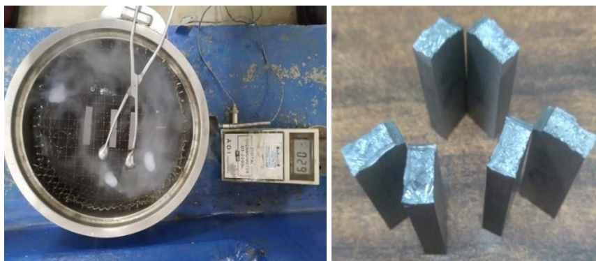
Figure 4.20 Charpy impact test (a) set up and (b) fractured impact test specimen
