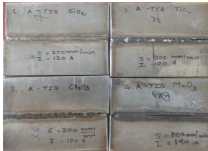
Figure 4.2 Welding current: 120 A, Torch speed 200 mm/min
