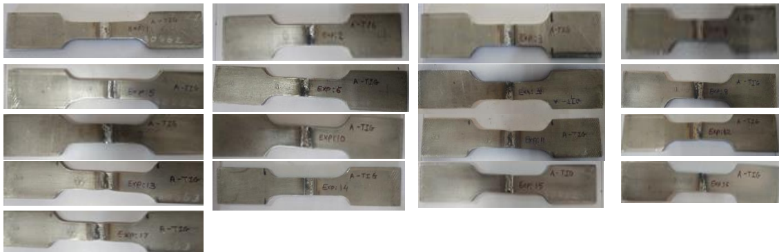
Figure 4.10 Failed tensile test specimen of A-TIG 2205 Duplex stainless steel weld
