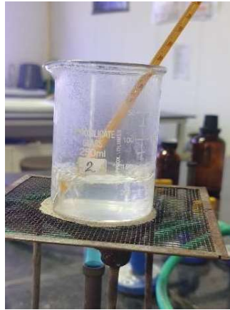
Figure 5-9 Boiling of CFF/PLA filament in 5% weight NaOH solution.
