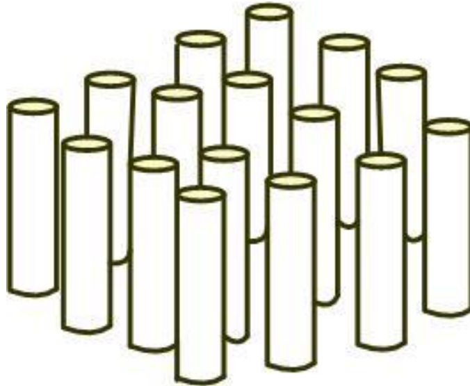
Figure 9.7: Pendry et al. presented a model consisting of conducting metallic cylinders to achieve negative permeability. (J B Pendry et al., 1999)
