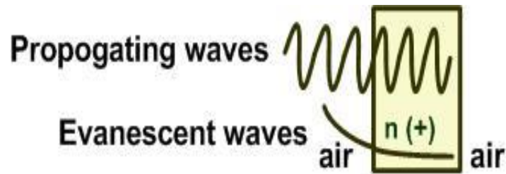
Figure 9.11: Propagating waves oscillate as Sine waves and evanescent waves decay exponentially.
