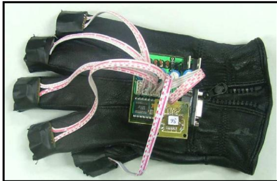
Fig.2.6: Sensing glove with six accelerometers and a basic stamp microcontroller proposed by Bui [13]
