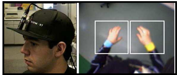
Figure 2.8: Head mounted camera and accelerometer data collection implemented by Brashear [18]
