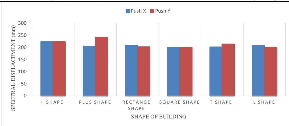
Figure 16 Graph of Comparison of Displacement
