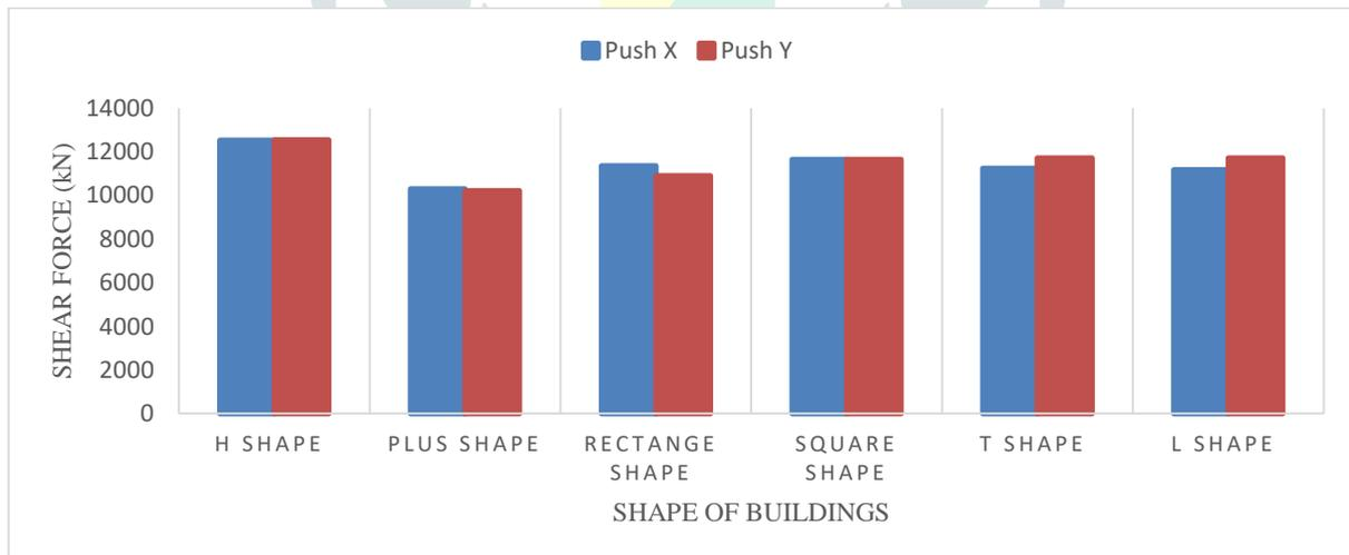
Figure 13 Graph of Comparison of Shear Force
