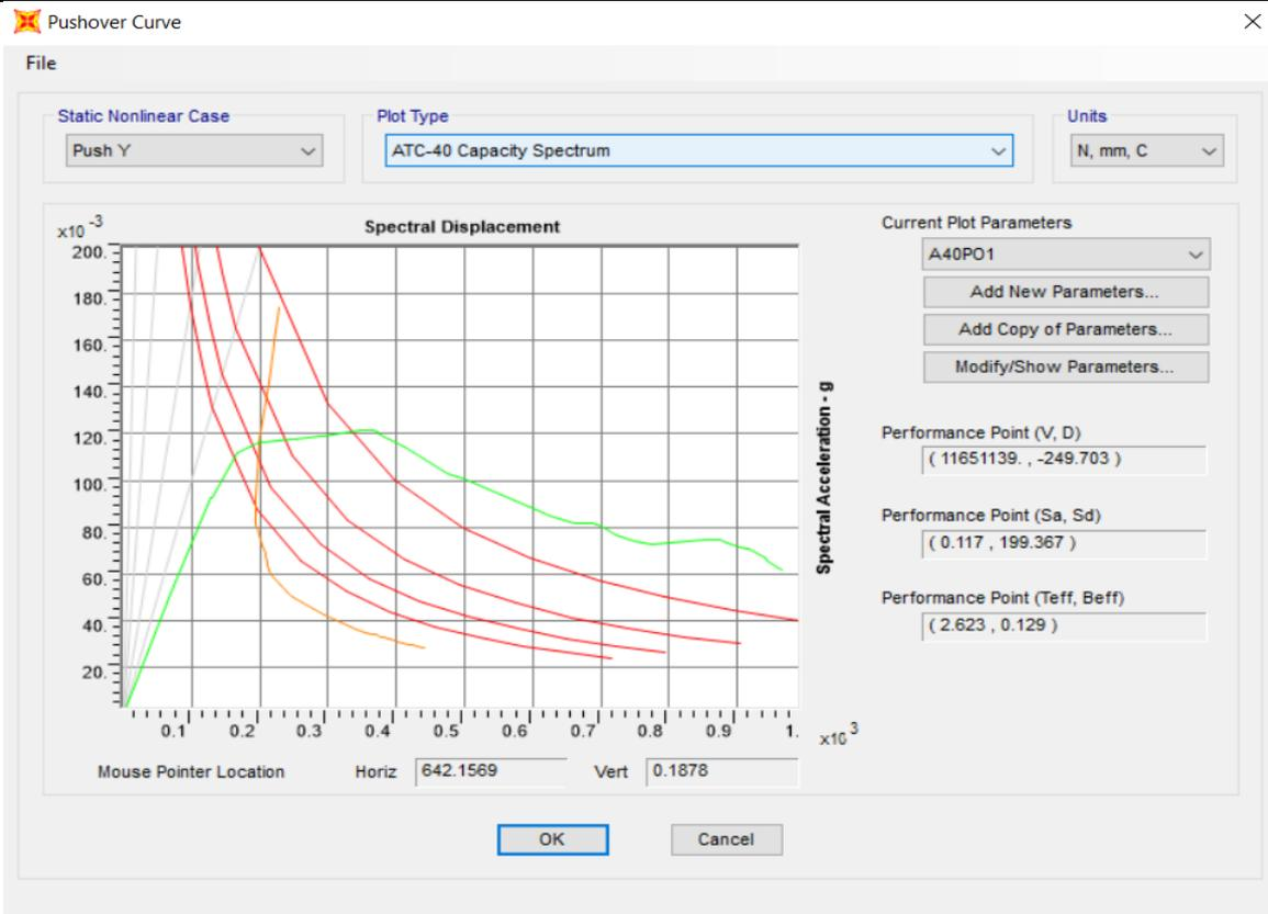
Figure 12 Capacity Curve for Push Y
