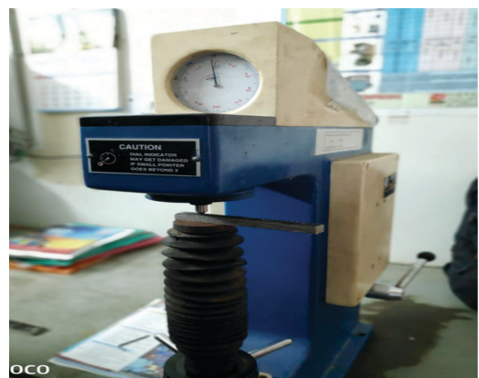
Fig. (12). Hardness test set up.
