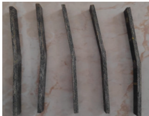
Fig. (10). Specimens after flexural test.
