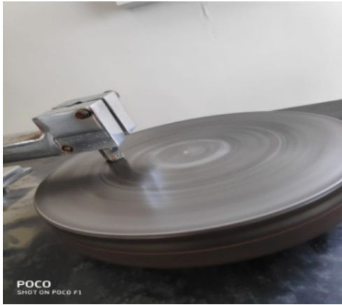
Fig. (13). Wear test on pin on disc setup.
