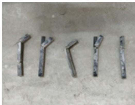
Fig. (11). Impact test on specimen.
