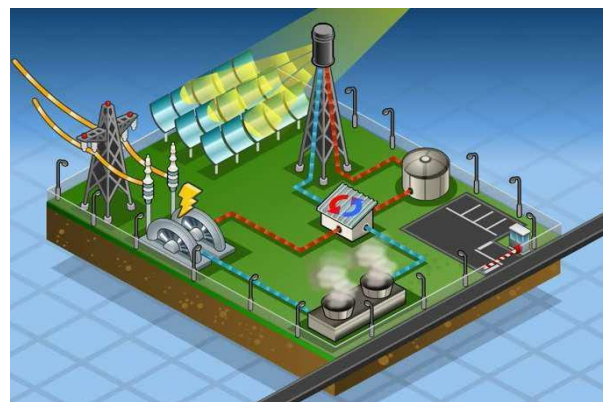
Figure III Basic CSP Plant
