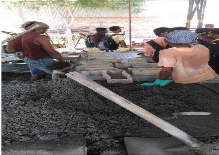
Picture 4.46 Students worked and prepared precast mold for a precast unit at the Precast manufacturing plant for assigned project practicums.
