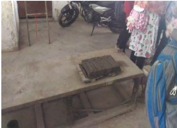
Picture 4.44 Students working on the precast mold for a precast unit at the Precast manufacturing plant for assigned project practicums.
