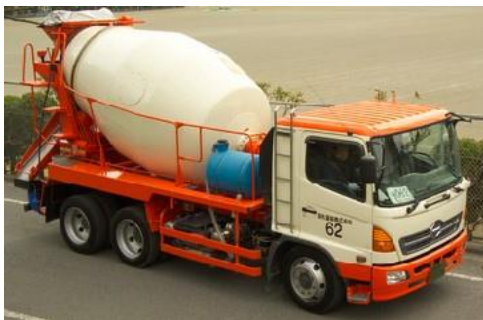
Picture 4.30 Concrete mixing transport trucks Source: theconstructor.org.
