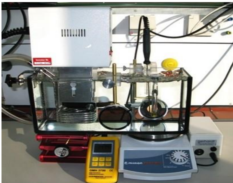
Figure 12. Pictorial representation of a thermostat water bath for phase studies of microemulsions (Anjum et al., 2009; Tessendorf, 2007).
