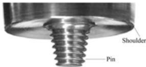
Figure 1.3 Friction Stir Welding Tool (Meilinger & Torok, 2013)
