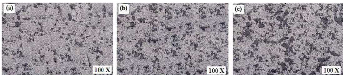
Figure 2.7 Microstructure of A356/SiC composites (a) 5% SiC (b) 10% SiC and (c) 15% SiC (Dwivedi, Sharma, & Mishra, 2014)
