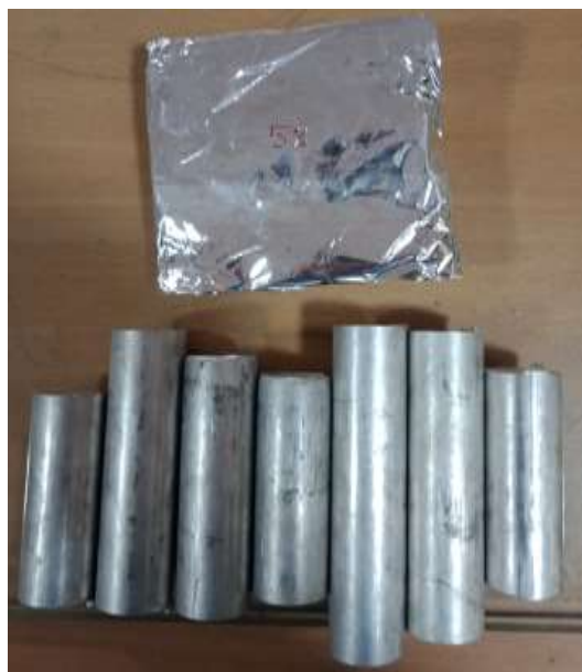
Figure 3.3 Aluminium alloy and wrapped SiC particles as per weight percent
