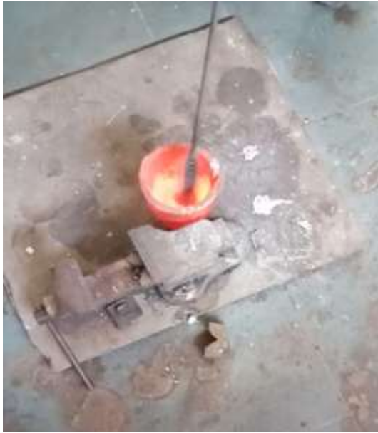
Figure 3.4 Formation of a vortex due to the stirring of molten composite
