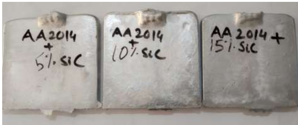
Figure 3.6 AA 2014+ x wt. % SiC Composite (x = 5, 10 and 15)
