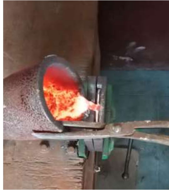
Figure 3.5 Pouring of molten composite in mould
